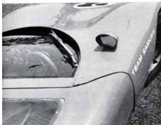
Radiator air exits through gap at base of windshield instead of usual outlet.
