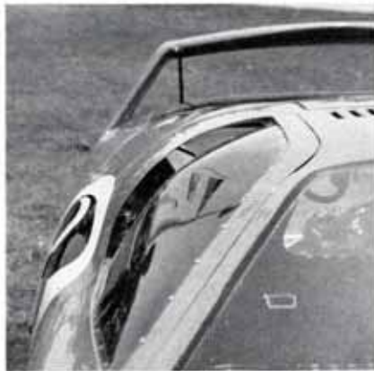
Compound-curved side window smoothly continues windshield curve to scoop.
