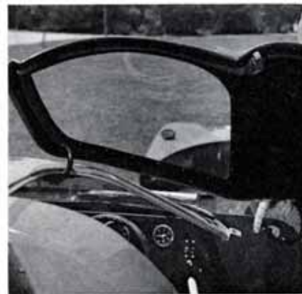
The unusual door-hinge arrangement. Tit-pin clips allow quick removal.
