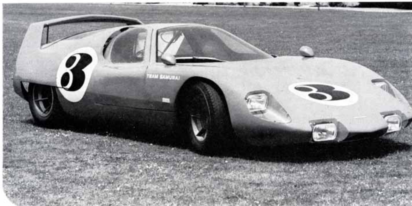
Brock's "ring airfoil" dominates the rear view.
